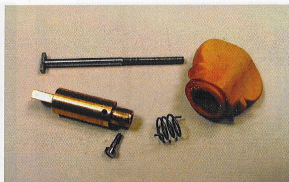
Extending mechanical key (modern reconstruction): key in pieces 3. [see also p10.]
