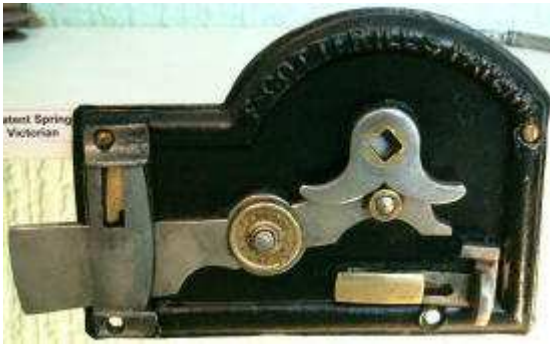
Improved door latch comprised in the 1846 Patent. It can be locked from inside the door by the bolt, bottom right
