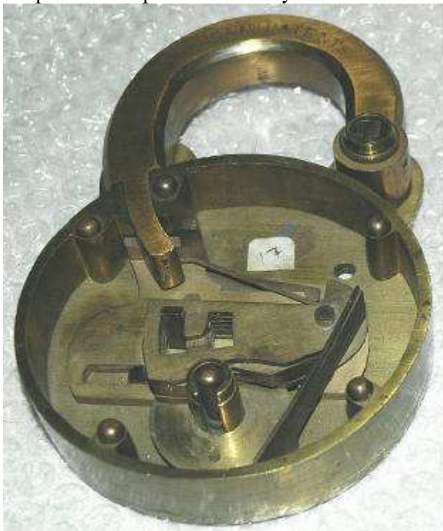
Hobbs Patent Padlocks , this first shown with its front cover plate removed to demonstrate the interior mechanism.
