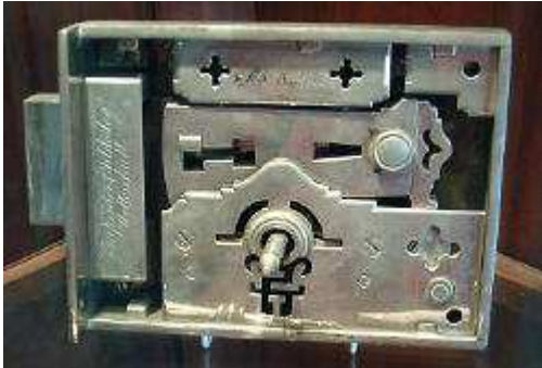
The Albert Lock, by Carpenter & Tildesley of Willenhall for the Great Exhibition of 1851 has elaborate wards, levers and a Bramah style lock mechanism.
