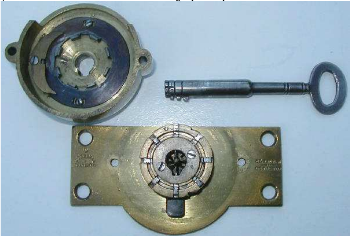
The ‘detector’ is the brass crescent moon shaped section of metal shown on the top left, and operates as described below:
