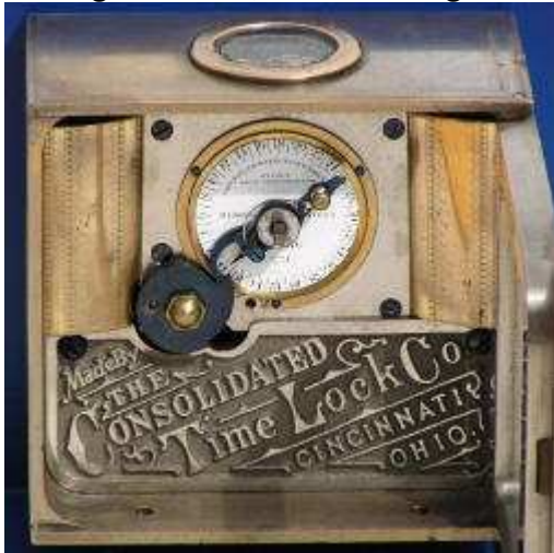
Consolidated Time Lock. 46 hour Single Lock Chronometer. H. Gross Patent.
