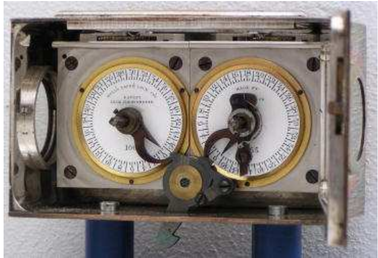
Consolidated's Double Time Lock stamped "Hall's Safe Lock Co's Patent Lock Chronometer" - another 46 hour lock.
